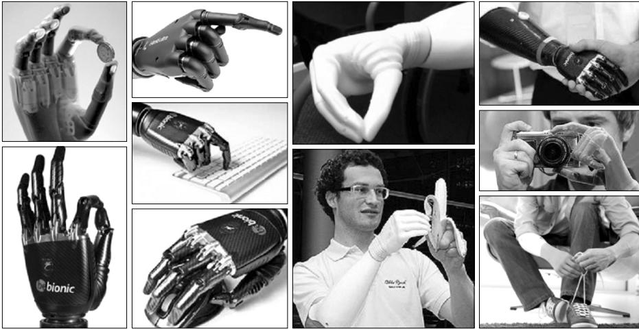
Fig. 6. Functions of the 5-finger type myoelectric hand prosthesis.
