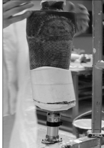
Fig. 24. Connecting the socket adapter.
