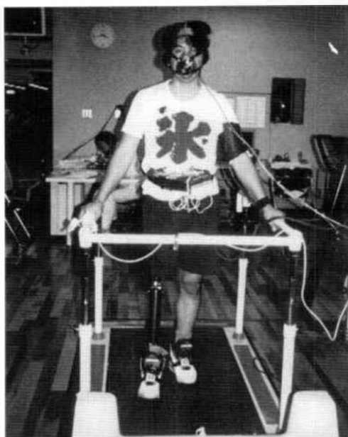
Fig. 1. Experimental subject undergoing respiratory gas analysis. Subject is instructed to hold the support bar lightly with both hands to avoid the danger of falling during measurement.
