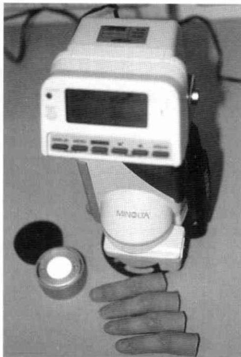
Fig 1. The spectrophotometric unit used for assessing the colour match results and the four prostheses which were prepared under illuminant TL84, F, D65 and a combination of TL84-F-D65.
