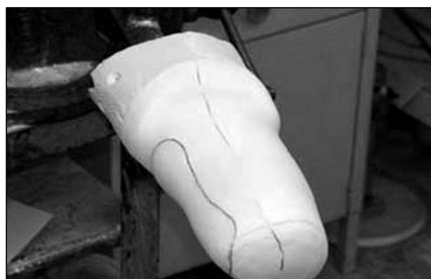
Fig. 12. Preparation for plastic sheets draping.
