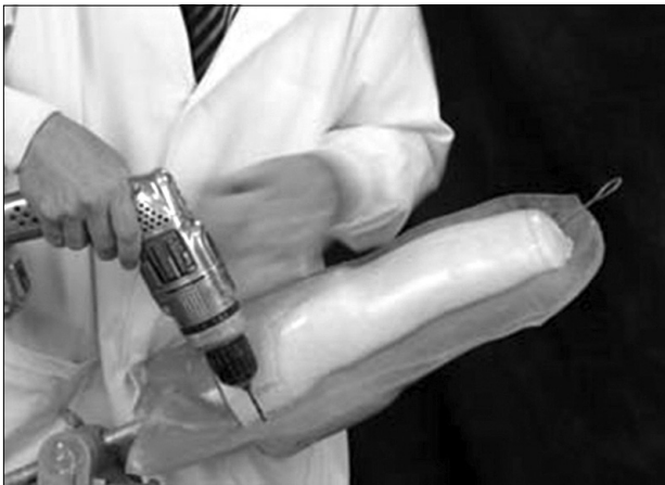
Fig. 14. Make the holes around model for clamp plastic sheets.
