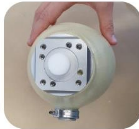
Use O-ring L-693112 to seal (cut to size)
